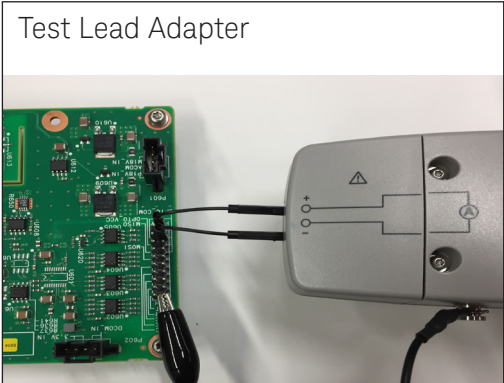
Figure 5. Connection of sensor head
