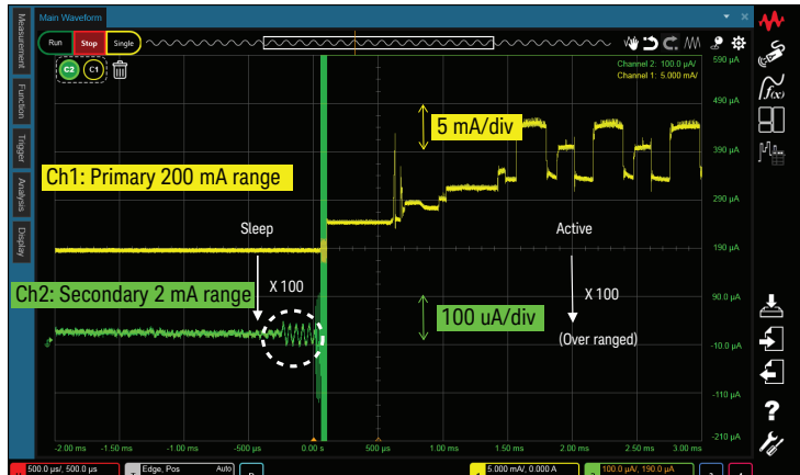
Figure 9. Current Profile Measurement Example with CX1102A Dual Channel Current Sensor
