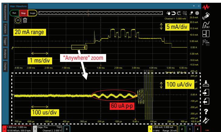
Figure 4. Zoomed waveform at the sleep mode of Figure 3
